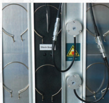
Four sensors monitor UV irradiance
